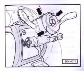
Release the locking lugs -arrows- and pull the reset ring off the steering column switch.
