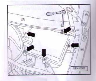
Remove the screws -arrows-from the protective housing in the reservoir and take off the cover.
