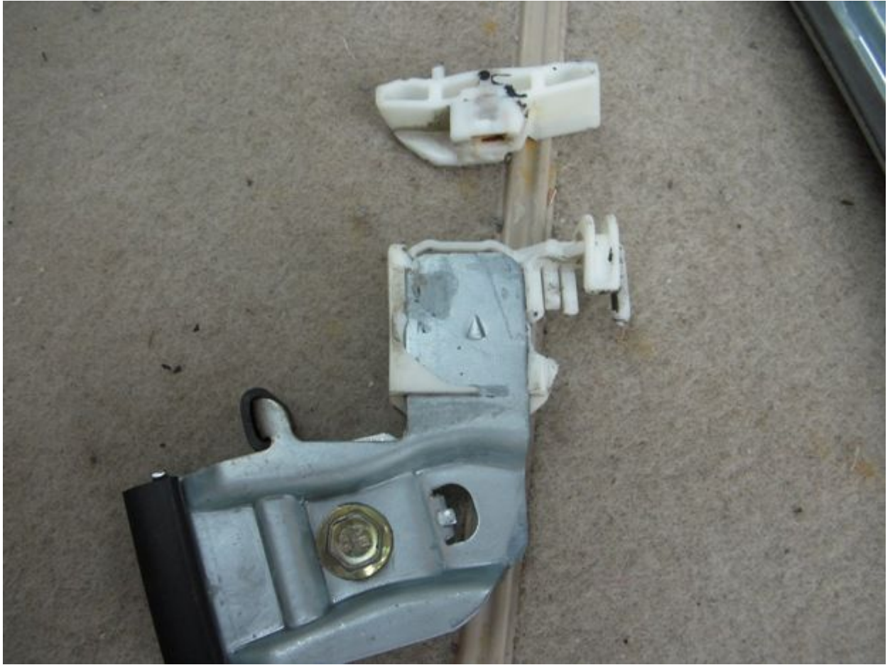
Back side of rear clip, showing where the cable hooks up:
