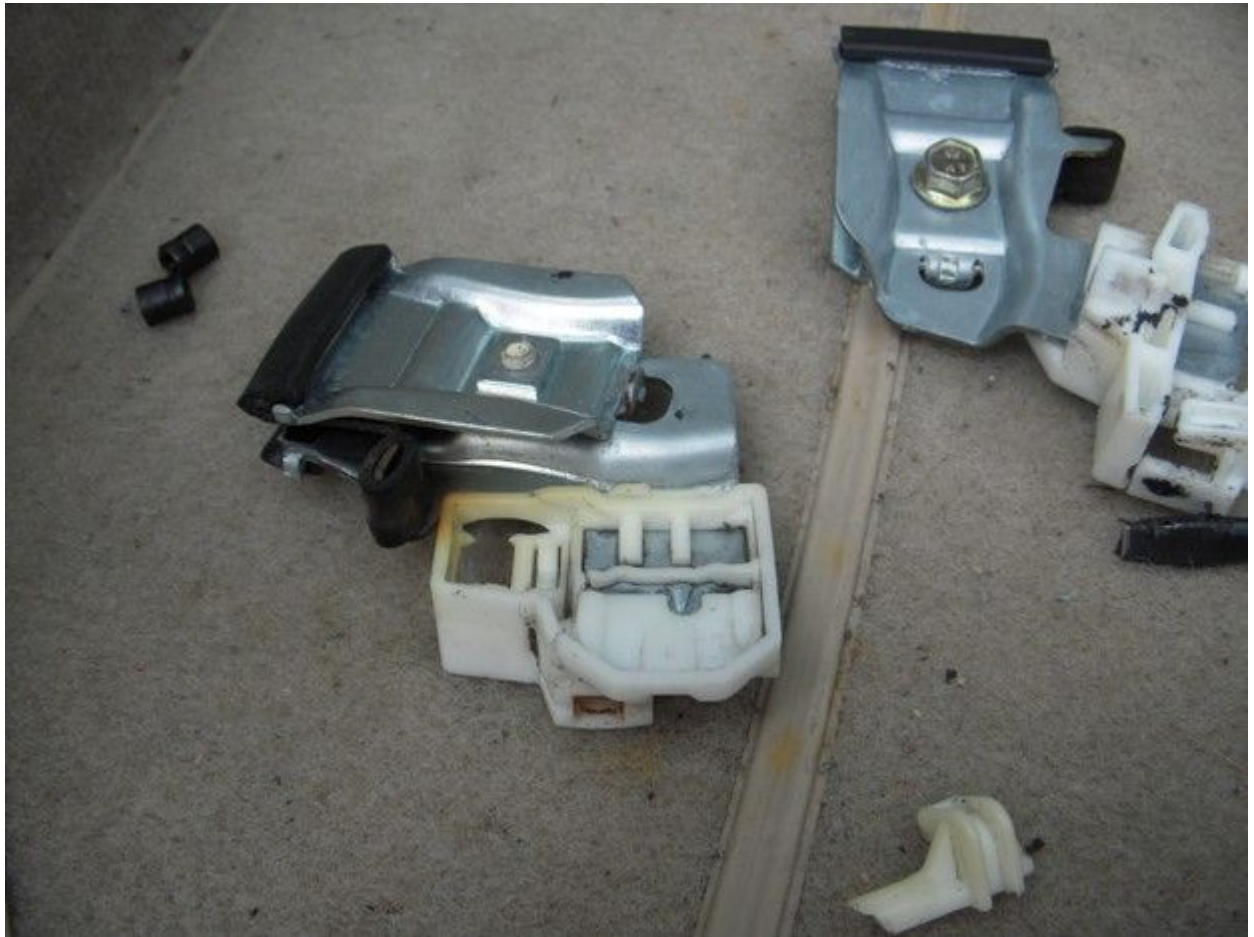
Rear clip, on arm but exploded, shows position of arm with respect to clip (look for triangular indent):
