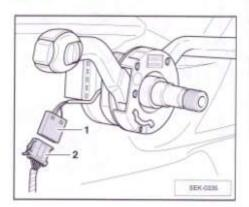
Connect the connector housing of the directional indicator switch with CSS
