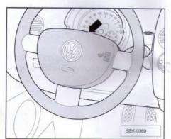
Remove the driver's airbag -arrow-.
