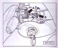
Disconnect both plug connections on the left side of the steering column switch -arrows-.
