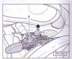
Remove the steering column switch
