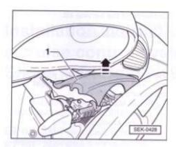
Remove the upper trim for the steering column switch -1- -direction of the arrow-.
