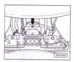
Remove the attachment screw -arrows-.
