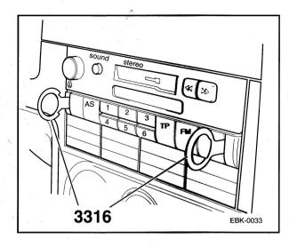
Insert Unlocking Tool VAS 3316 to unlock the radio navigation system, and then remove the radio/navigation system from the front.
