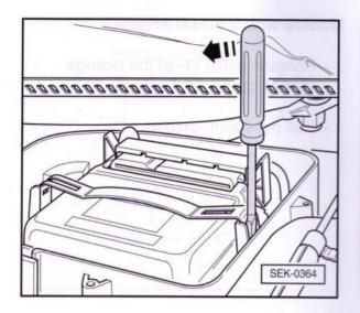
Remove the engine control unit after pushing the clamping collar in the -direction of the arrow- and unclipping it.
