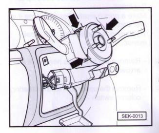
Release the locking lugs -arrows- and pull the reset ring off the steering column switch.
