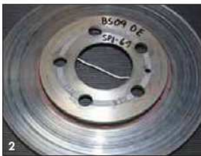
Figure 1. The 'other brand' brake disc in the second series of tests after 438 braking cycles. The disc has completely cracked.
