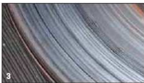
Figures 2 and 3. A Volkswagen original brake disc in the last series of tests after 440 braking cycles. Only light cracking is evident.
