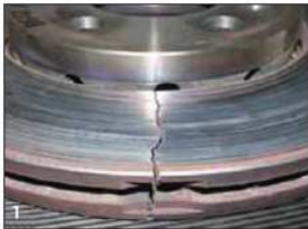
Figure 1. The 'other brand' brake disc in the second series of tests after 438 braking cycles. The disc has completely cracked.
